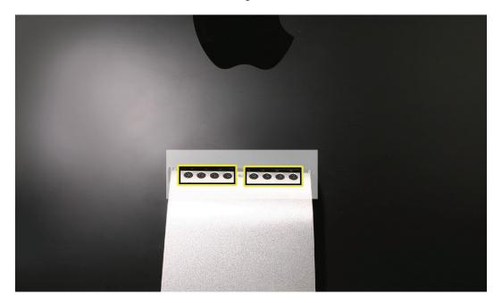
4. Separate the stand from the clutch mechanism and rear housing.
